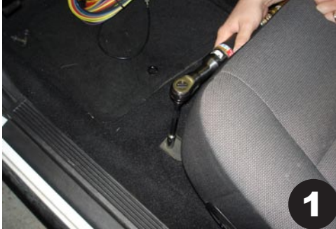
Use 9/16" socket to remove the front (2) seat bolts from the driver seat.
