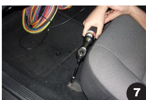
Use 9/16" socket to tighten (2) outside front seat bolts on the driver and passenger seats.
