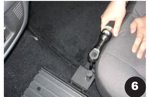
Slide floor plate legs into the correct position, anchor them to the inside seat bolts closest to the transmission hump.
