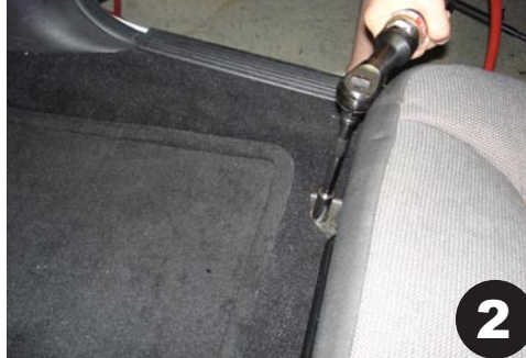
Use 9/16" socket to remove the front (2) seat bolts from the passenger seat.
