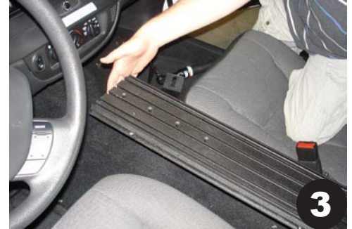
Set floor plate in-between seats.
