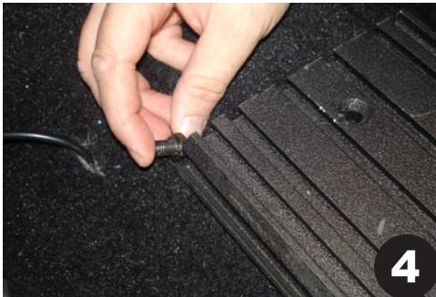
Insert (2) 5/16" bolts in each side of the floor plate side rails.
