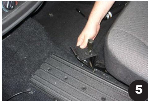
Attach floor plate legs to each side of floor plate with provided hardware, finger tighten nylock nuts to allow movement.
